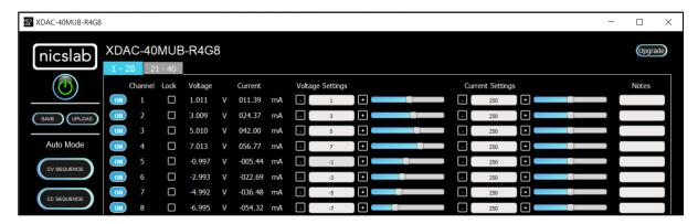
Note: When you upload CV mode, the current setting slider values automatically show 2184.50 bits to open the current flow from the supply. You may adjust this to match your requirements.
