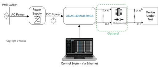
Figure 1. XDAC-40MUB-R4G8 System Diagram
